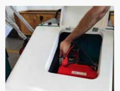
**EASY ACCESS TO THE BATTERY** The battery is located at the top of the machine and it is easily accessible and removable.
