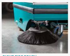
**RIGHT SIDE BRUSH** The right side brush is protected by the robust metal frame that help avoid any breakage caused by impacts during work.
