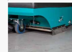
FLAP LIFTING DEVICE The flap lifting system is mounted on the front of the sweeper and allows the collection of bulky waste.
